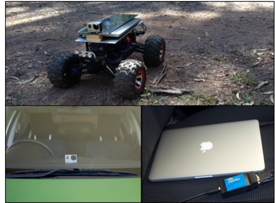
Fig. 4: Experimental setup, showing the RC car with GoPro camera and on-board laptop computer (top) and the road vehicle with GoPro camera (bottom-left), OBDPro and laptop computer (bottom-right).
