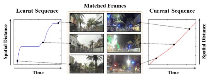
Fig. 1: Using condition-invariant, whole-image matching techniques and odometry, SMART compares image sequences with constant spatial separation between images.
