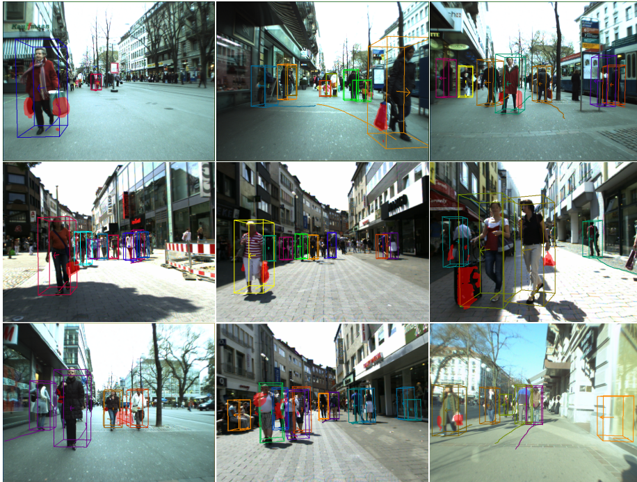
Fig. 10. Carried item detection results (in red). The bottom row shows some failure cases which are caused by depth smoothing, excessive body proportions, and unusually wide clothing.
