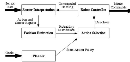
Figure 5: Navigation System Architecture
