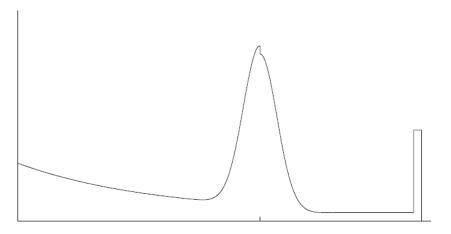
$$P(z \mid x, m) = \begin{pmatrix} \alpha_{\text{hit}} \\ \alpha_{\text{unexp}} \\ \alpha_{\text{max}} \\ \alpha_{\text{rand}} \end{pmatrix}^{T} \cdot \begin{pmatrix} P_{\text{hit}}(z \mid x, m) \\ P_{\text{unexp}}(z \mid x, m) \\ P_{\text{max}}(z \mid x, m) \\ P_{\text{rand}}(z \mid x, m) \end{pmatrix}$$
