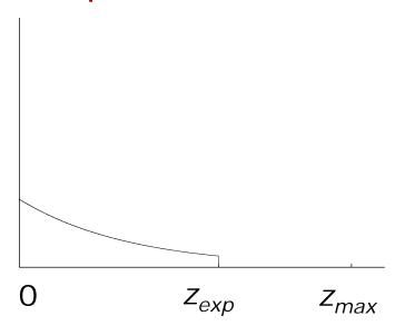
$$P_{hit}(z \mid x, m) = \eta \frac{1}{\sqrt{2\pi b}} e^{-\frac{1}{2}\frac{(z - z_{\exp})^2}{b}} \qquad P_{\text{unexp}}(z \mid x, m) = \begin{cases} \eta \lambda e^{-\lambda z} & z < z_{\exp} \\ 0 & otherwise \end{cases}$$
